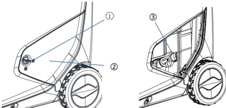
4. Refuel a recommended amount of oil and tighten the cap.
